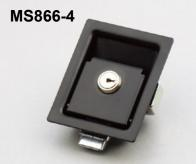
Main material and finish: Black powder coated steel cup and handle, sand blast and nickle-plated ZDC profile cylinder, zinc-plated steel latch, support and riveting screw Remarks: Default key K330
